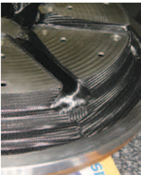
Unidirectional carbon fabric – fanning out from the spokes to join onto the rim – is being laid onto woven fabric layers underneath.
