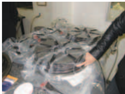
Moulds are placed into vacuum bags for 30 minutes, twice or three times during the layout process to compress/debulk the carbon fibre layers.
