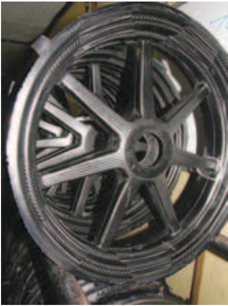
Wheels fresh out of the autoclave already have a very high quality finish.
